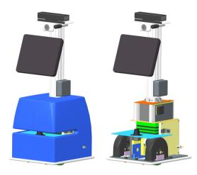
Fig. 2. CLARC robot prototype design
